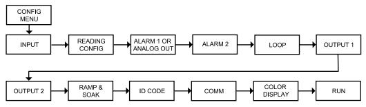
Figure 3.2 Flow Chart for Configuration Menu
